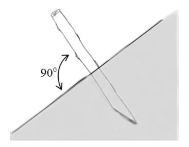
TYPICAL - Cut, Live Stake Insertion into Streambank Soil Profile.
